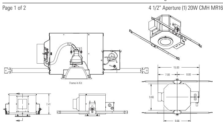
Ceiling Cutout: 5 1/16" (129 mm) Dia. Ceiling Thickness: 1 1/8" Max
